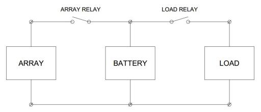
The MSRx Charge Controller provides connections for the Array Input, Battery and Load Output. It controls the Array & Load Relays to control the Battery charging and discharging.
